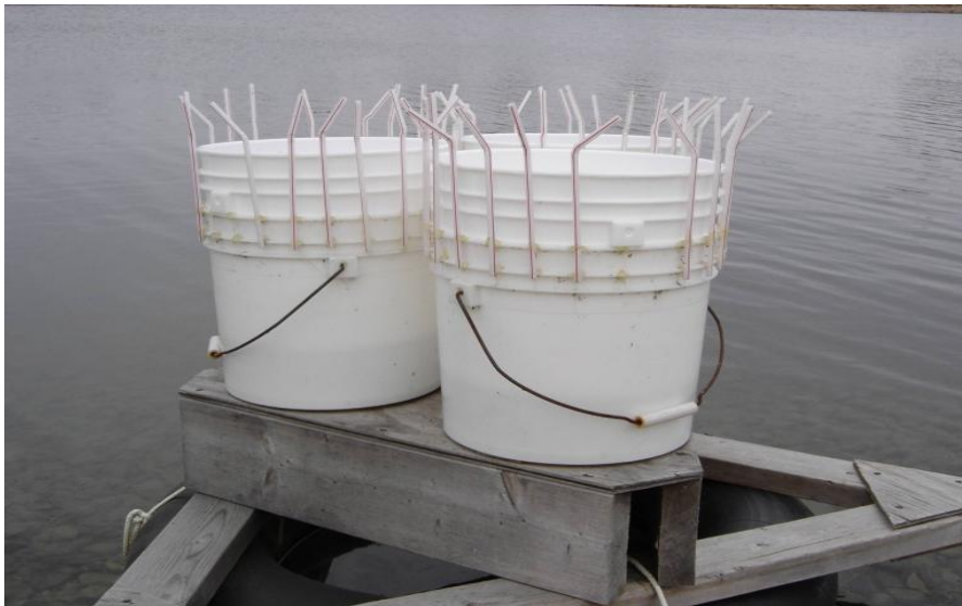
Figure 10: Bulk precipitation sampler.
