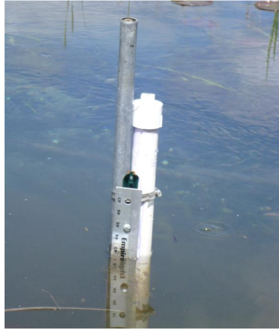
Figure 4: Stream-stage Hobo data logger.
