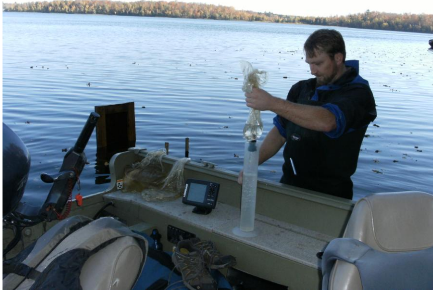
Figure 69: Andy Arens (ISWCD) measures shallow groundwater inflows to Pokegama Lake.
