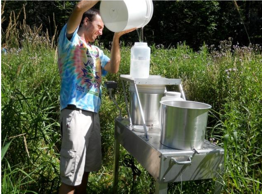
Figure 9: Ben Lakish (ICC Lab) and a wet-dry deposition sampler.
