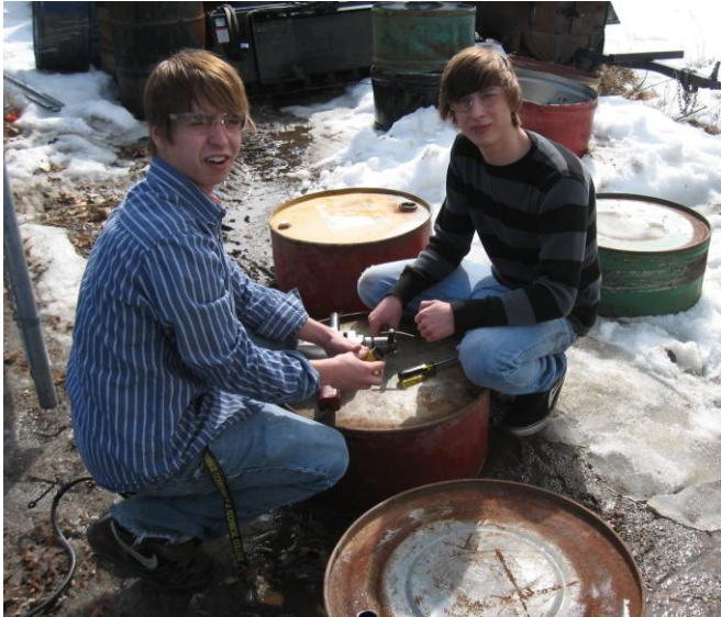
Figure 18: Students from Grand Rapids High School constructing seepage meters.
