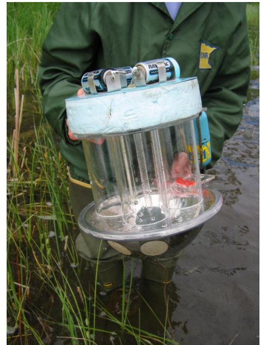
Image 8. “Night light” with invertebrates that are captured in the stainless bowl at the bottom.
