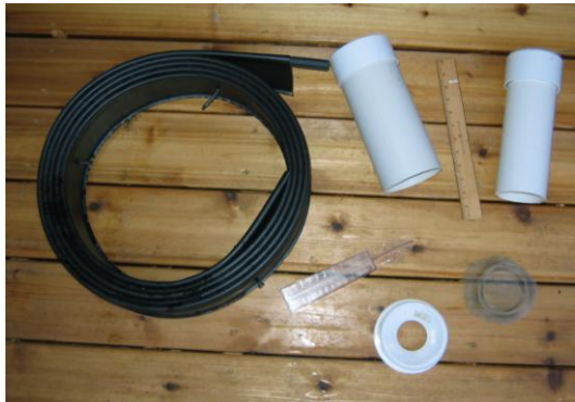
Image 1. Collectors were constructed from materials purchased at the local hardware store: (clockwise starting at upper left) lawn edging, 4” PVC with cap, (12” ruler for scale), 3.5” PVC with cap, screen to keep critters out, connector (used to funnel water into PVC tube) and rain gauge. Total material cost per collector: about $15.
