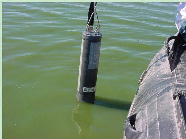
Water quality sensor being lowered into a blue-green algae bloom. photo John Downing
